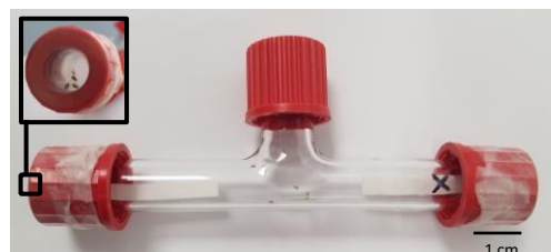
Figure 1. Olfactory two-choice bioassay tube. Groups of five aphids are placed in the center of the tube and have one day to choose the control side with ethanol-impregnated filter paper or the treatment side with a mixture of ethanol and EO and to settle on the artificial diet.
